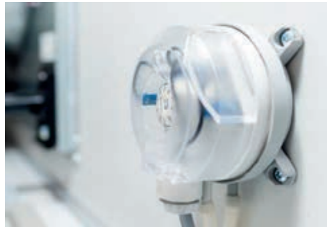
Differential pressure switch: effective measuring instrument to assess there is differential pressure across the filter and whether filters need to be replaced.
